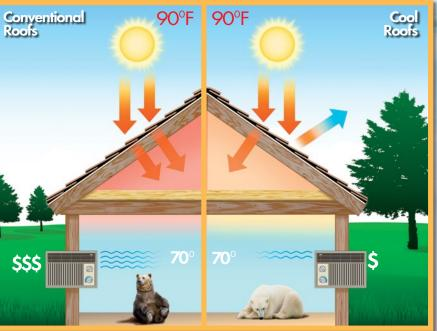
A cool roof from GAF helps minimize solar heat gain by reflecting incoming sun rays and re-emitting the absorbed energy - thereby reducing the heat going into the house and in the attic. This may translate into savings on air-conditioning bills."
